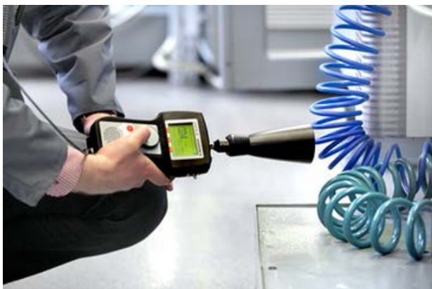
Ultrasonic leak detector helps identify CA leaks
