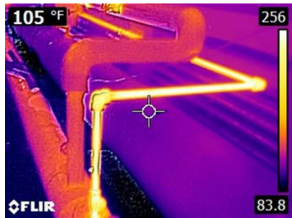
Thermal images taken during the study with visible high temperature, uninsulated piping.
